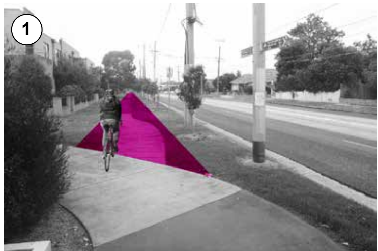
Back of kerb bi-directional path on Gordon Street.
