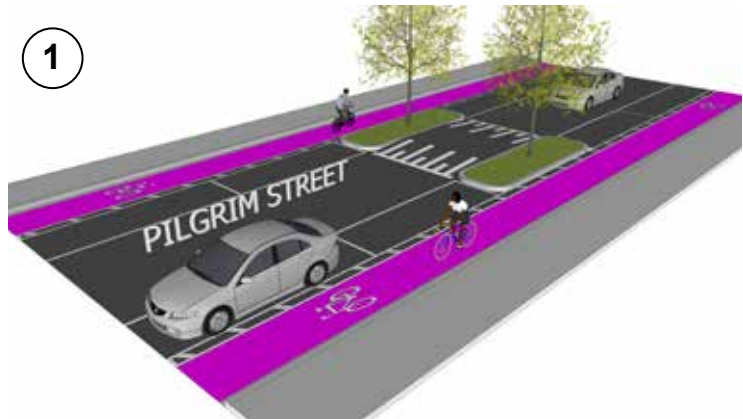
Lower motor vehicle speeds on Pilgrim Street with buffered bicycle facility 1.5m painted lane with minimum 6m buffer.
