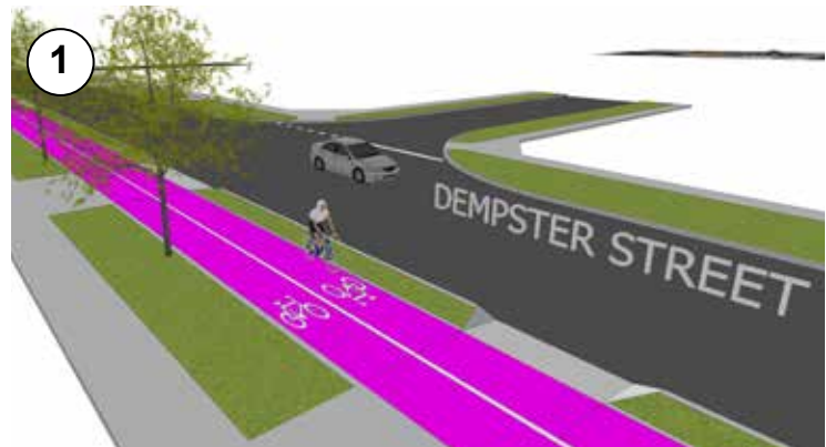
Off-road path from Tottenham Station – Extend kerb to accommodate bi-directional facility. Minimum width of bicycle lane 1.5m with planted buffer to kerb with minimum width of 0.6m.
