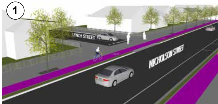
Extended kerbs on both sides of Nicholson Street. Minimum 1.5m raised bicycle lane with minimum 0.6m buffer.
