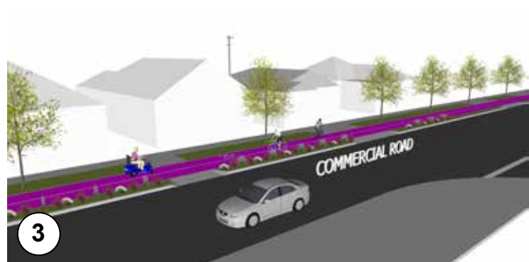
Extended kerb to create 3m bi-directional facility on Commercial Road with minimum 0.6m planted buffer.
