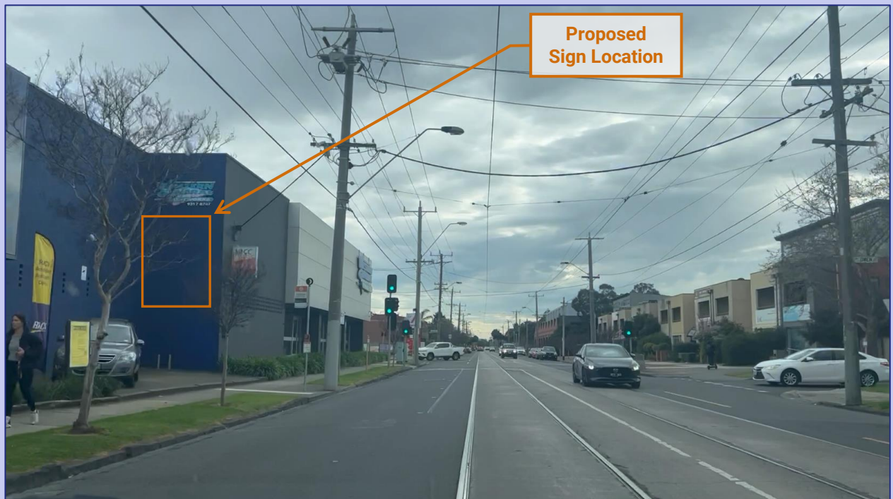
Figure 12: Northbound approach – sign passes outside drivers' 20° cone of reading vision (25m to sign)
