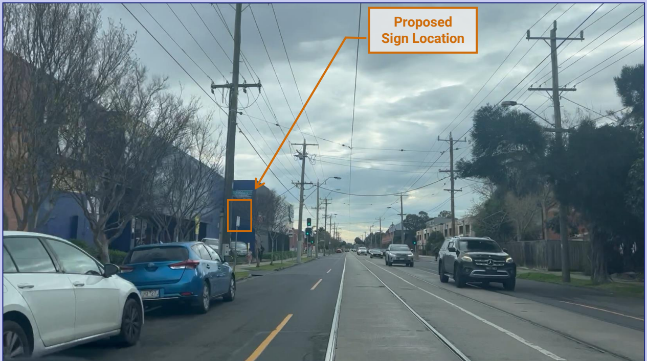
Figure 11: Northbound approach – sign first visible, passes outside drivers' 10° cone of reading vision (55m to sign)
