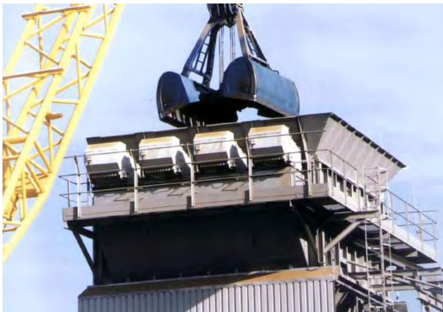
Figure 6: A hopper comparable to that proposed with the dust extraction systems visible on one of two sides, and with material being dumped into it from a crane operated grab bucket.
