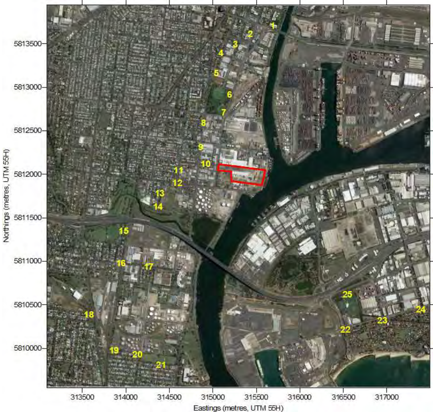
Figure 1: Local area around the existing cement plant site, surrounded by industrial land use, with numbered receptors representing the nearest sensitive receivers comprising residential areas and sporting fields. Receptor 10 is representative of the nearest dwellings along Frederick Street within the Industrial 3 zone.
