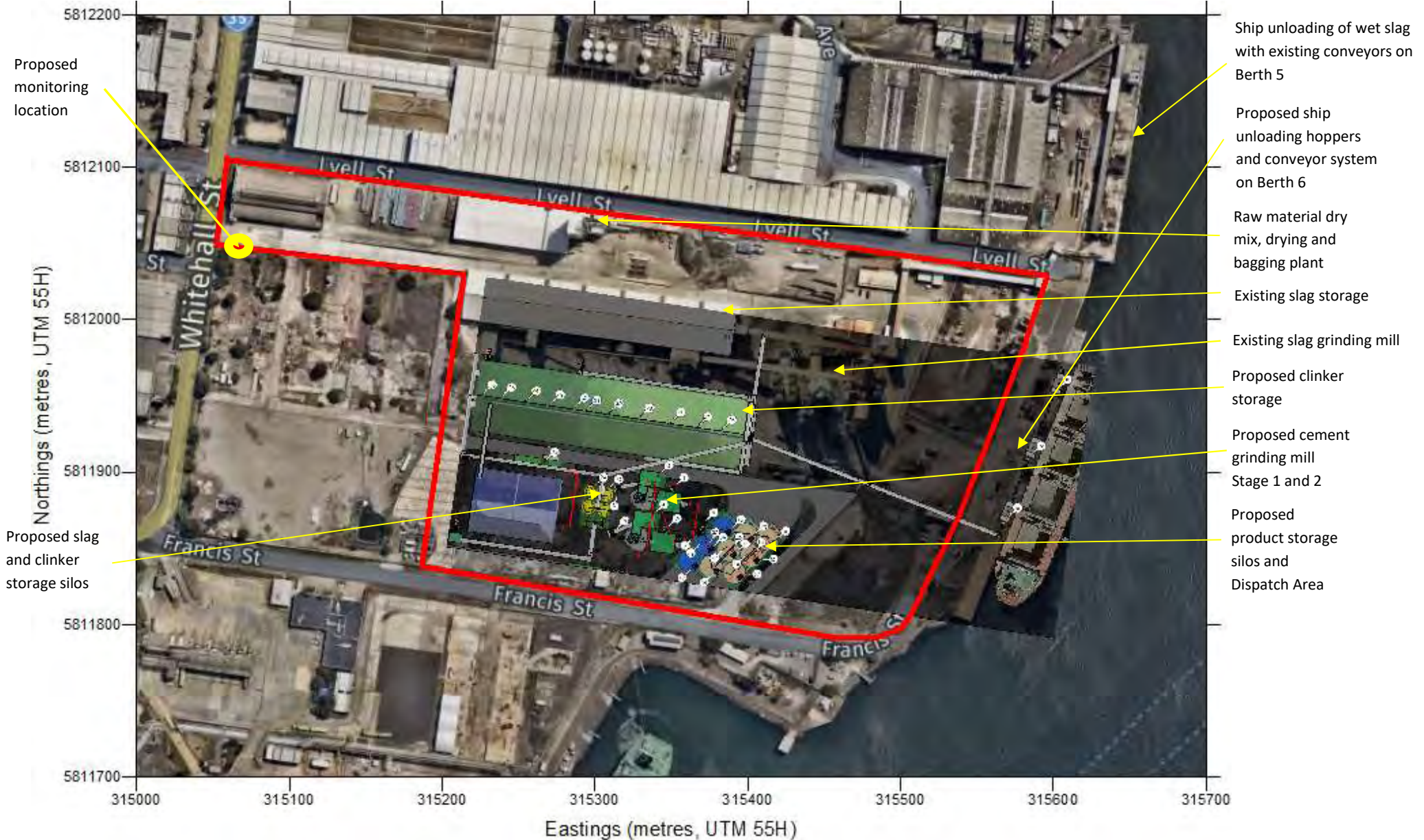
Figure 2: Site area with features of the proposed additional and existing plant indicated, as well as the proposed monitoring location near the western boundary.
