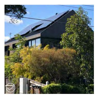
Location and provision of solar panel should be decided at the beginning to ensure they are integrated in roof design.
