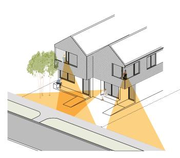
Habitable rooms and balconies along the street provide activation and passive surveillance that increases the sense of safety.
