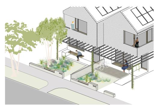
Entry verandah or porches form an important component of the dwelling connecting the outside with the inside. They should be designed to provide sufficient standing room and weather protection.
