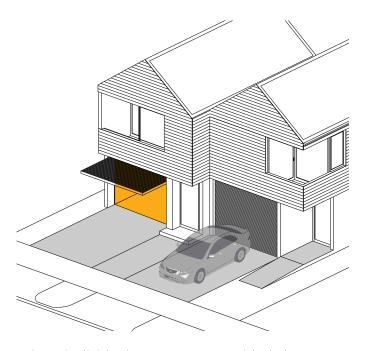
Where individual garages are provided, they should be designed to have natural light and ventilation so they are adaptable for alternative use if not required as a garage.
