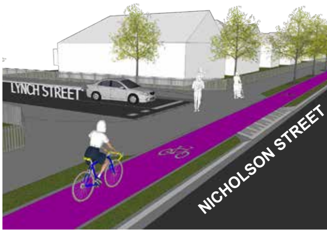
Nicholson Street protected cycle lanes concept Kerb extensions and raised thresholds will prioritise cycling along Nicholson Street without the removal of existing street trees
